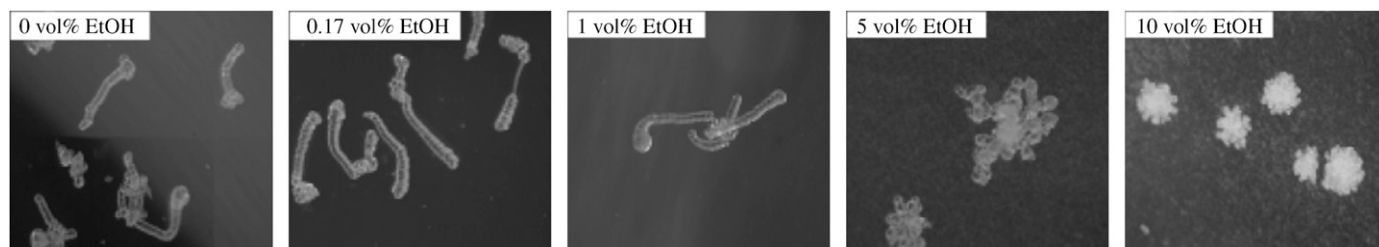
Fig. 4. Optical micrographs of self-assembled silica-carbonate at different EtOH vol%. [TEOS] = 7.5 mM, [Ba 2+ ] = 5 mM, pH = 11, T = 20 °C, and t = 9 h.
