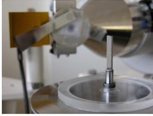
Figure 1: A core sample of 7.5mm x 7.5mm cross section mounted on the tomography rotation stage before imaging.
