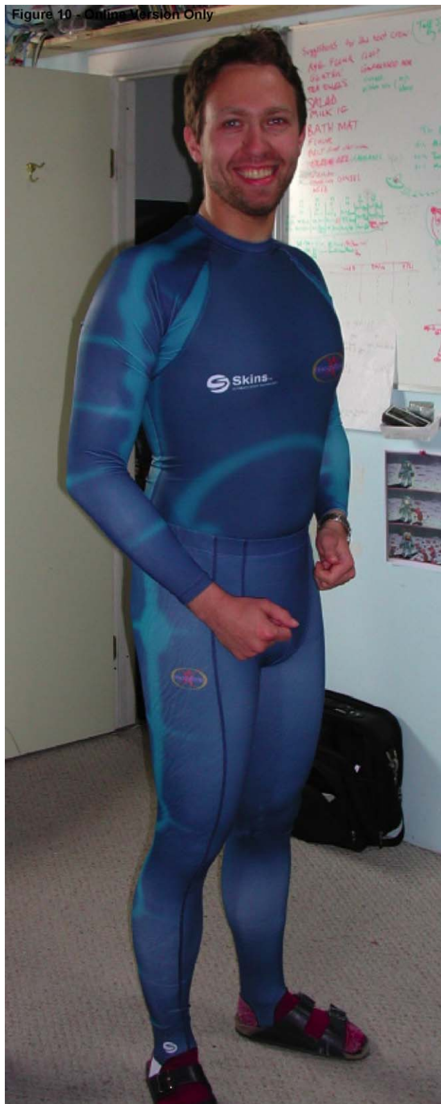
Fig. 10. The analogue MCP layer of the MarsSkin analogue space suit, which is made from a poly-lycra coolmax material with sublimation printing and simulates the compression of a real MCP garment.
