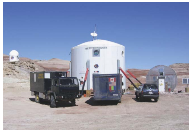
Fig. 12. Three low-fidelity pressurized surface vehicle prototypes under test at the Mars Desert Research Station in Utah during Expedition One (Persaud et al., 2004). From left to right are the Everest Rover, the ARES Rover and the Sports Utility Vehicle (SUV) used.
