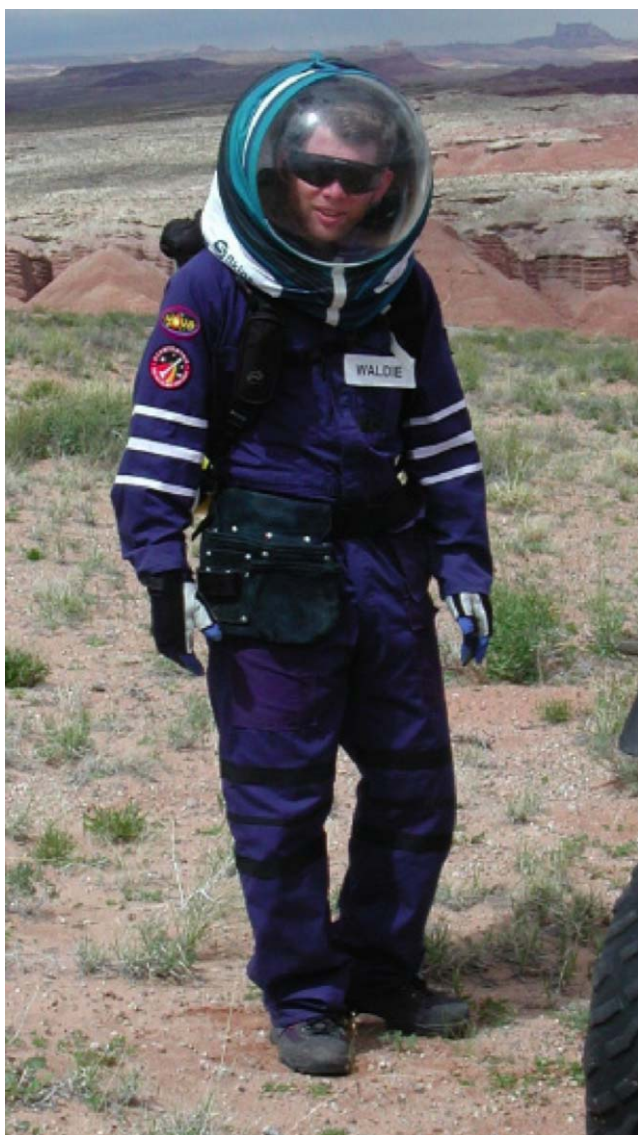
Fig. 8. A front view of the MarsSkin analogue space suit showing the helmet assembly, the outer protective layer and the utility belt.
