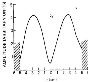
FIG. 5.—Radial variation of the components of the wave fields,  $b_r$ ,  $b_\theta$  and  $b_z$  for  $B = 33$  G. The solid curve for  $b_r$  and  $b_\theta$  is a theoretical fit for  $ak = 0.63$  and  $\Omega_e\tau = 3$ ; the broken curve has  $\Omega_e\tau = 300$ .
