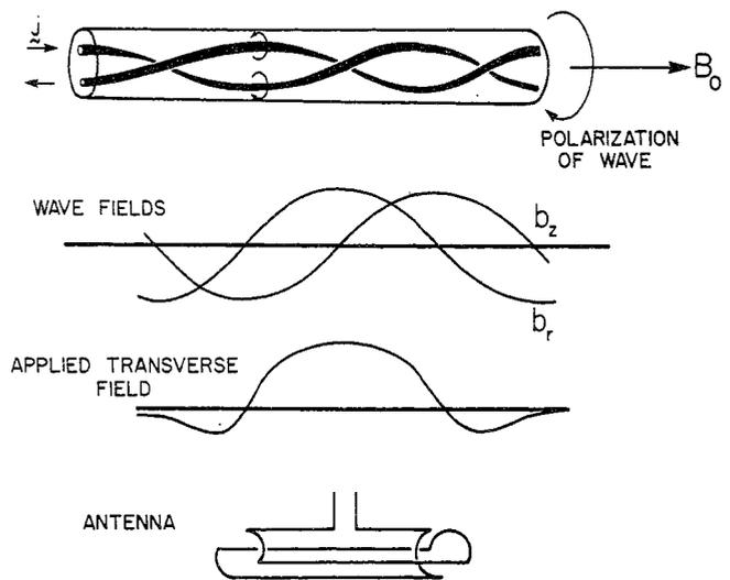
FIG. 2.—Sketch of the current system for an  $m = 1$  helicon with associated wave fields (a, b). The exciting antenna and its applied transverse field are shown in c and d.
