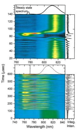
FIG. 2 (color). Typical data showing soliton explosions. In the upper panel the dispersion is adjusted to yield solitary explosions, while in the lower it is adjusted to yield bursts of explosions (see dispersion curves in Fig. 1). The resolution and position of spectral channels has been optimized in the lower panel.
