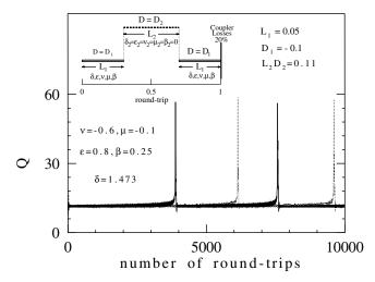
FIG. 3. Soliton explosions in numerical simulations. The soliton energy Q is plotted versus the number of round-trips. Q corresponds to the experimental integrated intensity. Parameters of the simulation are shown. The inset shows the map of the parameters of the CGLE for a single round-trip in the laser as used in our numerical simulations.
