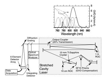
FIG. 1. Experimental setup. The radius of curvature (ROC) of the laser mirrors are indicated; those not designated are flat. The graph shows a typical steady state spectrum, the spectral response of the individual channels (dashed line), and the dispersion as a function of wavelength. The dotted dispersion curve corresponds to upper panel in Fig. 2 while the dot-dashed curve corresponds to the lower panel.
