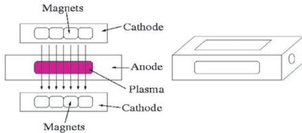
Figure 2. Schematic of the PD for He metastable production.
