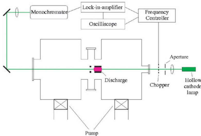
Figure 3. Experimental setup for the investigation of metastable He atoms.
